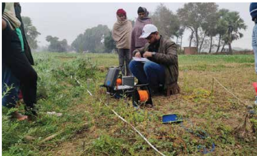
Hydrogeophysical Survey Vertical Electrical Sounding for underground layer information at Kujap Panchayat, Nagar Block, Gaya ji District, Bihar
